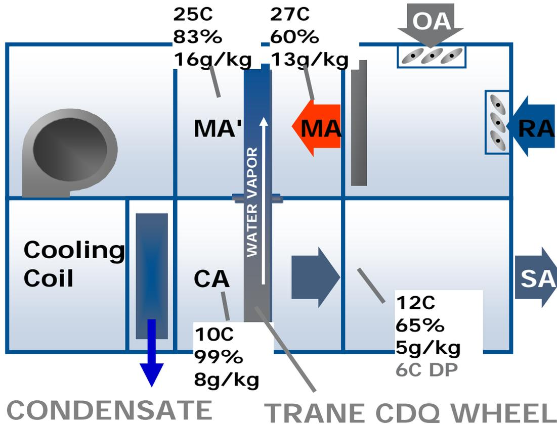
CDQ can produce supply air with dew point lower than the coil chilled water temperature or refrigerant suction temperature
