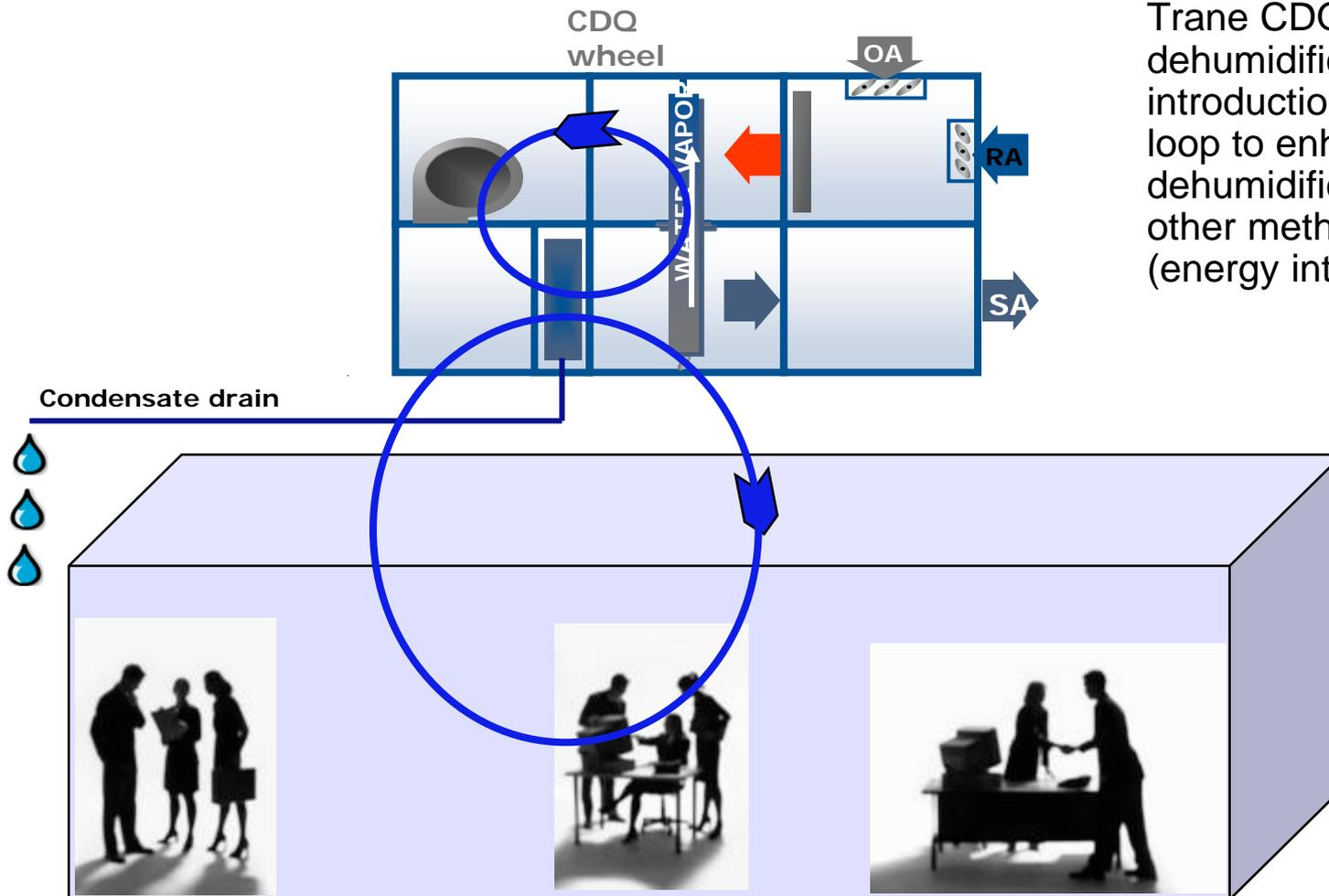
Trane CDQ's primary dehumidification method is the introduction of 2nd moisture loop to enhance cooling coil dehumidification. This is unlike other methods that uses heat (energy intensive).
